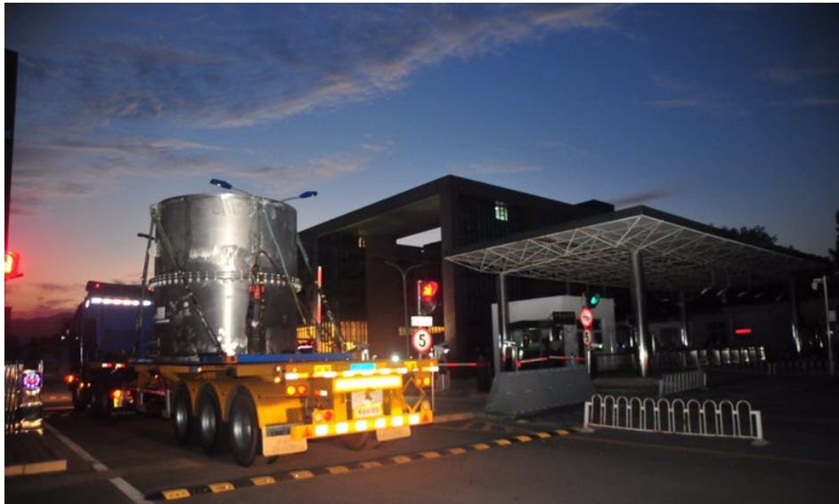
Figure 11. Ghana micro-reactor HEU spent fuel transportation
